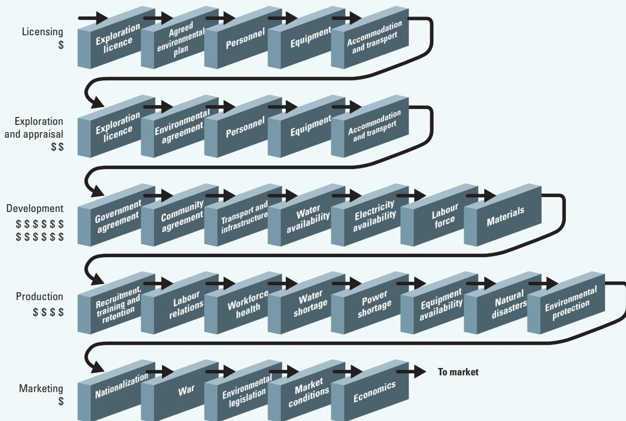
Schematic illustration of the possible barriers to be overcome in order for a project to move from an exploration idea to a mine that is delivering material to the market place. Failure to negotiate any of the barriers could lead to project failure. Dollar signs are an indication of the level of expenditure associated with the related stage of a project.
